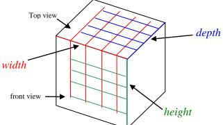
orthogonal to both. By projecting the spacing along the dimension out to the right onto the line representing the side view we locate the widths for that view. By projecting the spacing along the heights of the front view onto the line representing the side view plane, we locate the heights for the side view.
